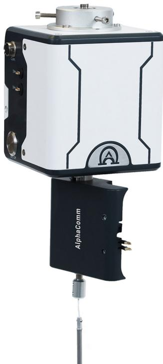
**AlphaComm** is a motorized slip ring commutator with the ability to control the sensitivity and velocity of the motor, and to eliminate signal noises that are caused by undesired animal movements, all in a simple setup.
